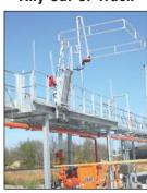
Track mounted gangway can be moved back and forth along the elevated track and extended as necessary to provide safe and easy access or egress from the vehicle no matter what the spotting or configuration.
