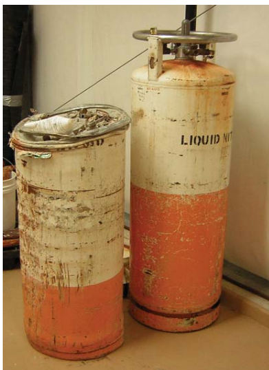
Intact cylinder and remains of a ruptured cylinder
